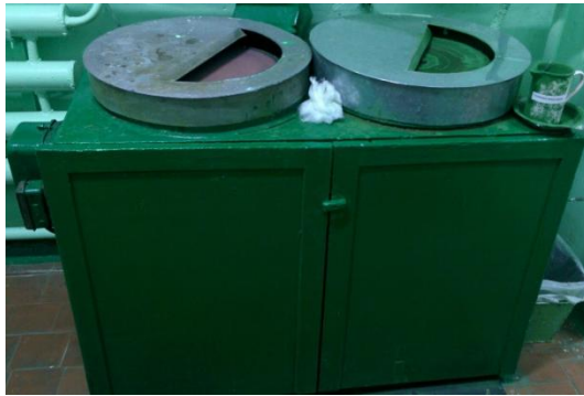
Figure 2 – Self-made grinding and polishing machine A new method for polishing samples
