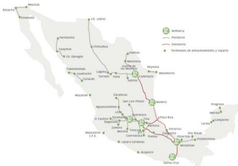
Map of transport and distribution of curd and derivatives to refining centers and storage terminals: 1) Refinery 2) Pipeline 3) Pipeline 4) Storage and distribution terminals
